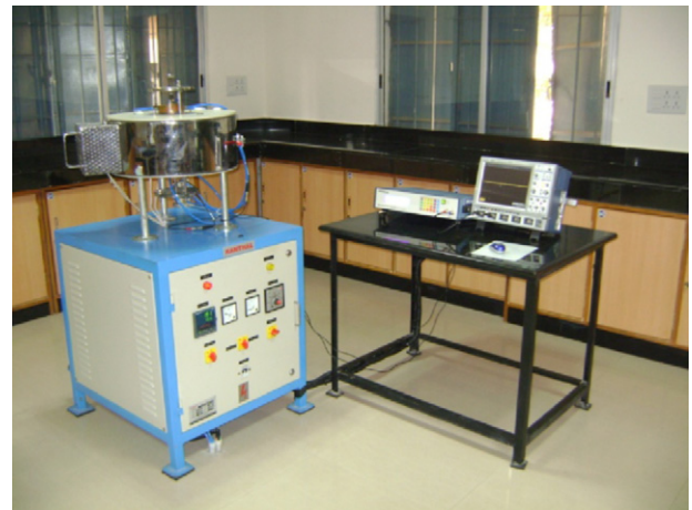
Fig. 2. Experimental arrangement for on-line ultrasonic velocities and attenuation measurements over a wide range of temperatures.
